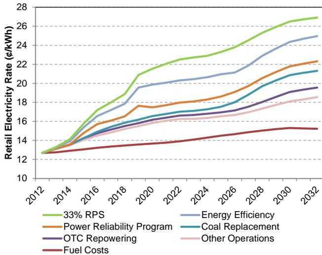
**Figure 2:** Incremental rate impacts of LADWP costs and initiatives over the next twenty years. “OTC Repowering” refers to retrofitting of coastal power plants that employ inefficient once-through-cooling using ocean water; “Power Reliability Program” refers to basic infrastructural upgrades like pole and transformer replacement.<sup>4</sup>
