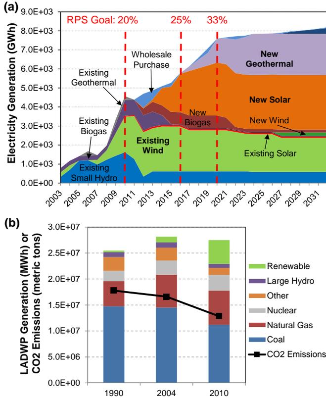
**Figure 1:** (a) LADWP renewable energy generation, historical and projected. “Existing” sources refer to those in operation by 2012, while “New” sources will be constructed subsequently. RPS milestones are delineated in red and the major portfolio components to meet the 33% RPS target are listed in bold.<sup>4</sup> (b) LADWP total historical electricity generation broken down by source, with carbon dioxide emissions overlaid.
